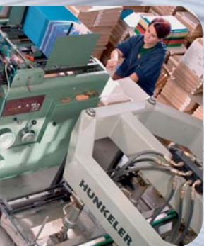
Inner books are automatically inserted into the ready-made book covers
